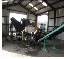
The shredding of tires started in 1988. Employees de-rim tires on site and recycle the rims. Tires are then processed through the tire shredder. The finished product is used as supplemental daily landfill cover, and used in drainage projects, pipe substrate and to repair seeps.
