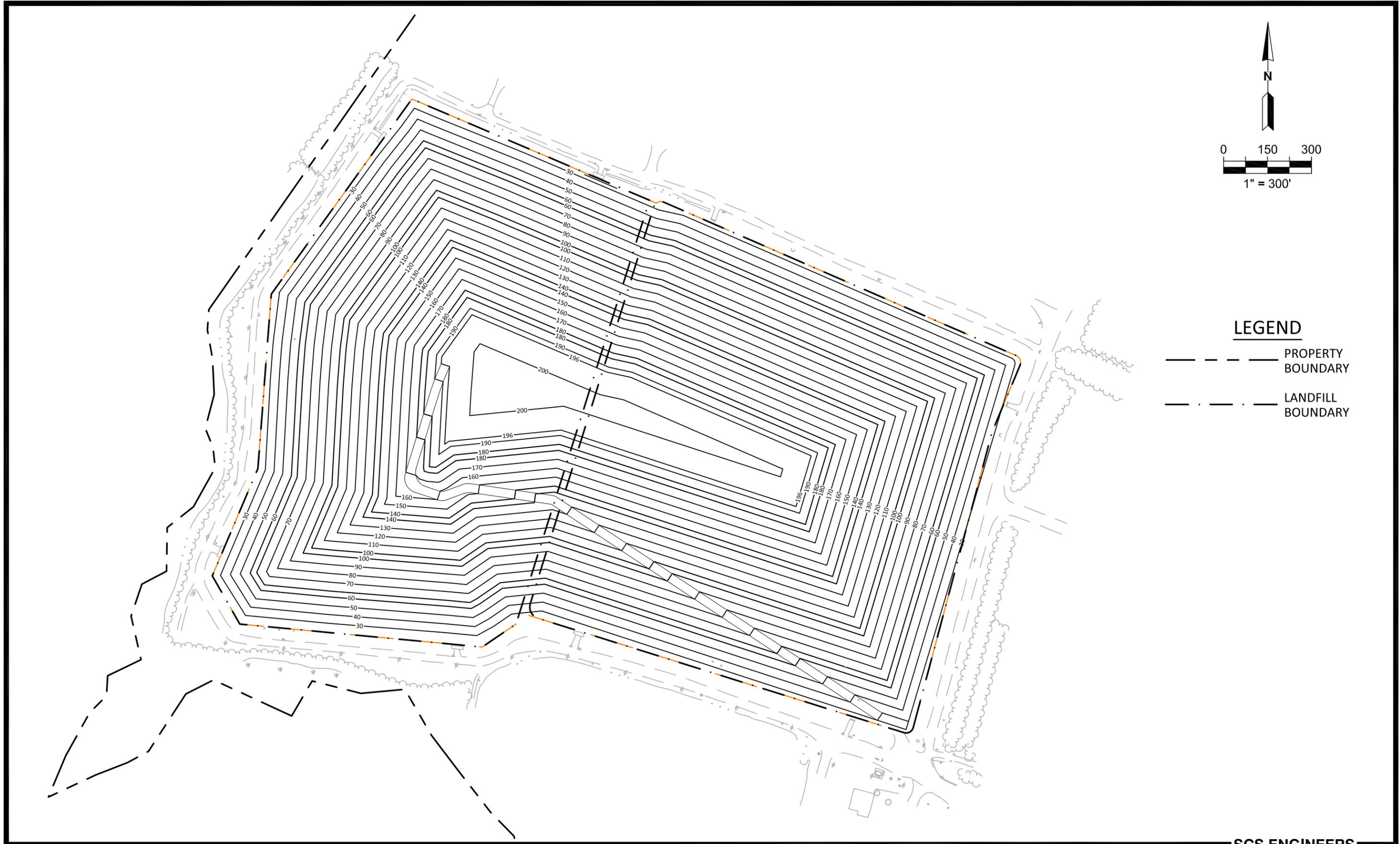
FIGURE 3. CELLS V AND VI PERMITTED TOP OF WASTE GRADING PLAN
