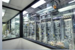
Laboratory scale reactor stations that can be configured as fixed-bed, trickle bed or continuous stirred tank reactors (STR).
