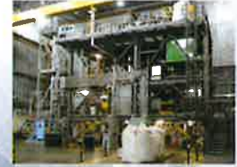
Full commercial scale tubular (fixed-bed) FT reactor at TRI's demonstration facility in Raleigh, Durham, NC.
